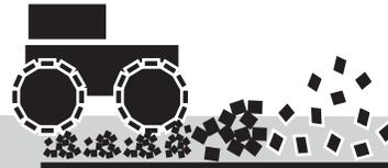
The garbage is compacted to make room for more trash to be dumped until the landfill reaches its capacity.
